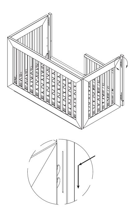
**NOTE:** MAKE SURE RAILS ARE LOCKED IN PLACE BEFORE MOVING TO NEXT STEP
